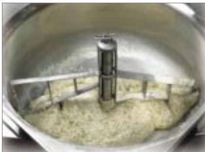
Proveno kneads dough in a matter of minutes (mixing programme number 6). In-kettle proving. (Tempguard: proving control).
